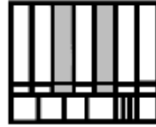
Fig. D. When adjusting hue (tint) on a monitor that displays blue only, these two bars and the patches under them should have the same intensity.
