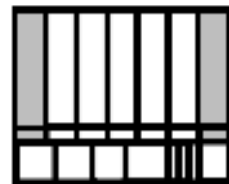
Fig. C. When adjusting color (chroma) on a monitor that displays blue only, these two bars and the patches under them should have the same intensity.
